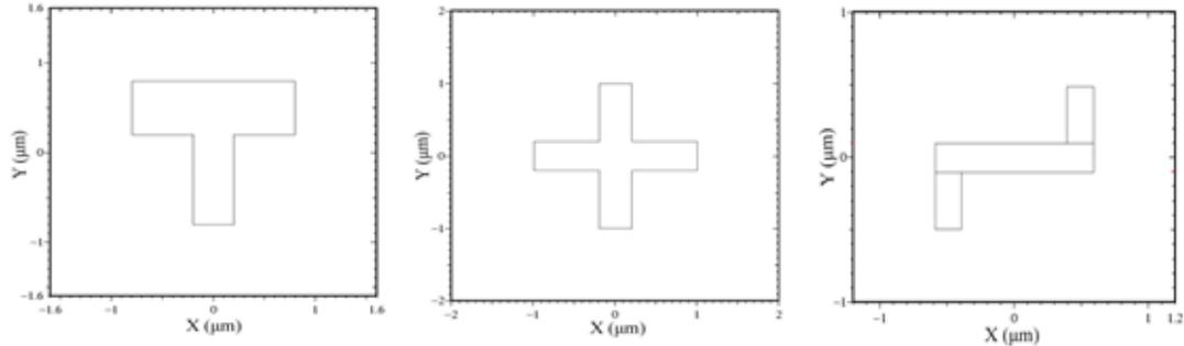
Figure 1: Three testing layout patterns before OPC. The line width of the right figure is equal to 180 nm.
