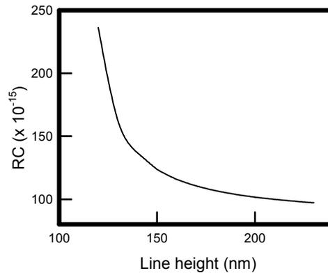
Figure 6: RC time delay of the RE-shaped interconnects with different line height.
