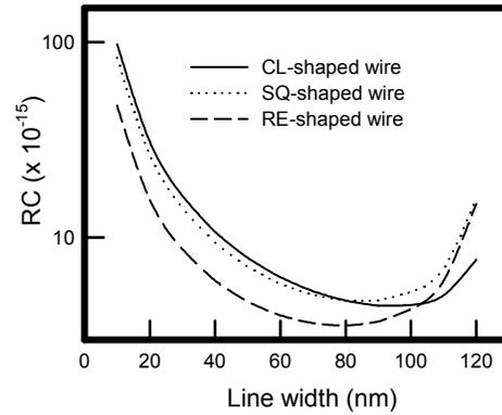
Figure 5: The RC time delay calculated for the three interconnects with different line width.
